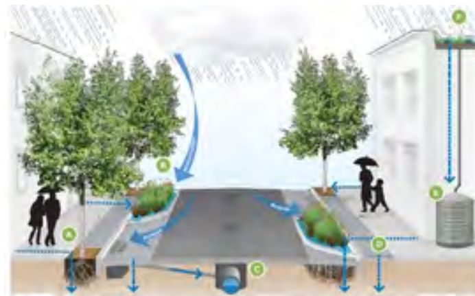
(A) street trees with flow through planters (B) rain gardens (C) upgraded sewer pipes (D) permeable pavement (E) cisterns (F) vegetated roofs
